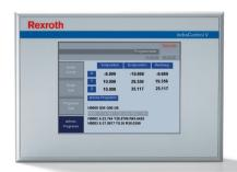
These controller-based compact operrator terminals allow you to edit your production data simply by pressing a key or touching the screen. The system versions cover a range from simple small graphics displays to touchscreens with full graphics capabilities – with the number of function keys depending on the system design. The comprehensive interface range fulfills almost all of your communication wishes, whether Ethernet TCP/IP, field-bus or serial.
