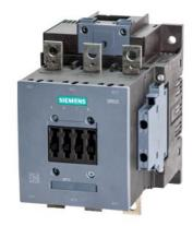
Contactor 220 ... 240 V AC/DC AC3 55 kW 400 V AC (50...60 Hz) / DC operation auxiliary contacts 2 NO + 2 NC, 3-pole, size S6 with box terminals conventional operating mechan. screw terminal
