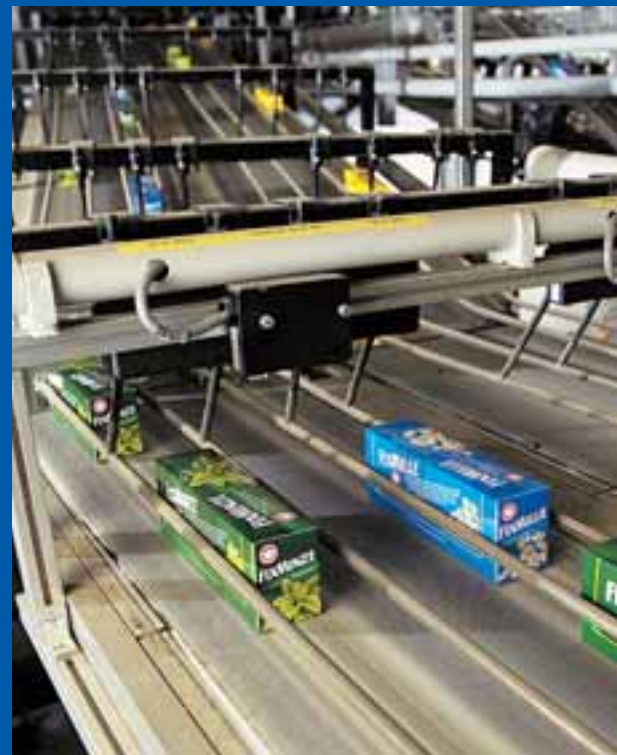
Lenze 8200 vector frequency inverters have been used in this packaging system. Communication takes place via PROFIBUS DP.
