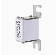
Fuse-link, high speed, 400 A, AC 690 V, DIN 00, aR, DIN, IEC, single indicator, live gripping lugs
